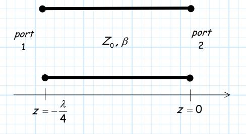
Using the **definition** of admittance parameters, evaluate this 2-port device and find explicitly the values  $Y_{11}$  and  $Y_{21}$ .
